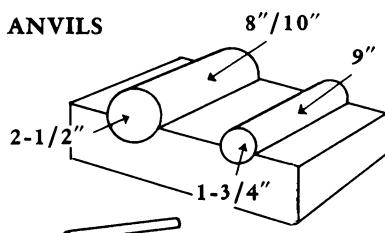
Footnote: Indentations in holder must be lined with soft felt to obtain maximum of resonance. To obtain resonance hit both tubes simultaneously with beater (small piece of tubing) held by the middle. Damping is obtained in the same fashion but keeping the contact with the two tubes.
